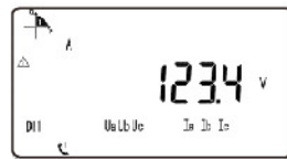
Voltage on A phase
